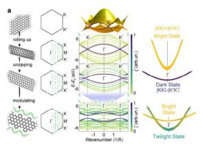
We have recently demonstrated a dramatic improvement in the optical properties of graphene nanoribbons by the use of chemically synthesized ribbons which have a well-defined structure and width. Adding a regular side chain to the ribbon creates a one dimensional superlattice and strongly inhibits aggregation. As a result, we see narrow excitonic ZPL (Zero Phonon Line) emission from thin films as described in our latest work (Sturdza et al, Nat.
