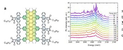
Figure shows the nanoribbon structure (left), and the temperature dependence of Micro-PL from 1 micron spots of a high density (right) film of GNR deposited onto silicon substrates
